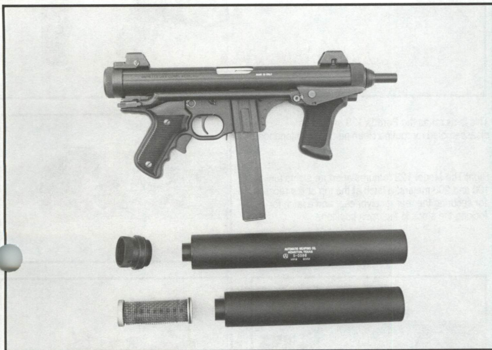
The AWC MK-9 suppressor (top) has a mount for the Walther MPL and MPK submachine guns, while the shorter MK-9A can has an Uzi mount. The separate rear end cap and thermal diffuser convert either suppressor to fit the Beretta 12S. These specialized end caps actually replace the barrel-retaining nuts on the respective submachine guns.
